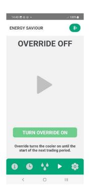
Press the Override button to bring the cooler out of standby to allow for additional cooling to take place when trading hours are unexpectedly extended.
