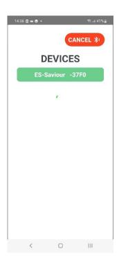
Press the Red BLE button to scan for devices then select the device you wish to connect to.
