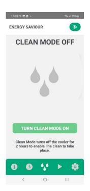
Press the Clean button to put the cooler into standby for a couple of hours to enable the cleaning process to take place.
