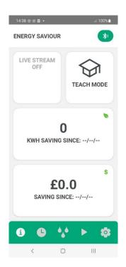
Track your energy saving from the app. Select an option from the menu at the bottom of the screen. Note savings will not be displayed until the unit is running in Normal Mode
