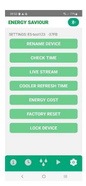
Press the Settings button to bring up the available options. Live data will give a value of line voltage and the connected cooler power consumption in real time. The lock function can be set so that the settings cannot be adjusted without unlocking the device first. Keep a note of the code.
